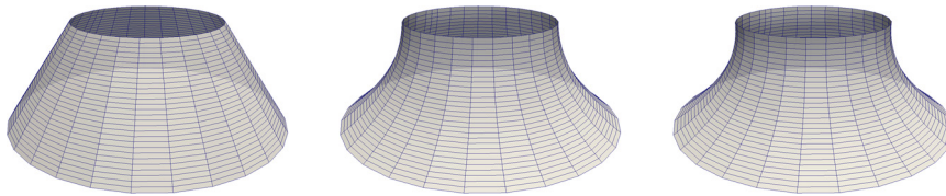
Fig. 3. A catenoid approximation is also obtained (cf. Fig. 2) if Algorithm 2 is applied to an initial truncated cone. The sequence illustrates the initial surface followed by the first two iterations. The third iteration (not shown) is indistinguishable from the second to the naked eye. In this simulation the initial cone dimensions are: upper radius 1.6, lower radius 3 and height 3. The spline space used is periodic of degree 3, with 30 knots in each direction. Similar order of convergence as of Table 4 were also obtained in this case.
